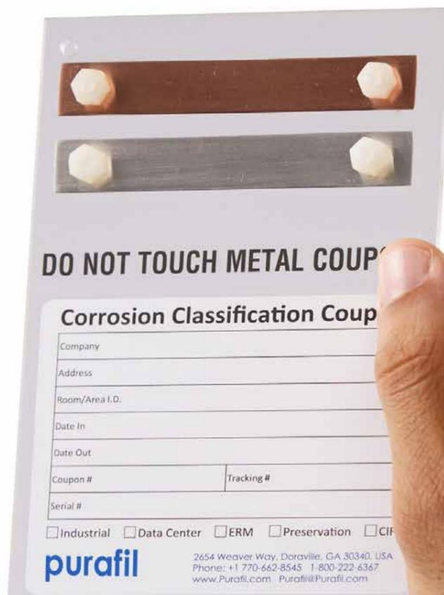
Purafil Corrosion Classification Coupon
