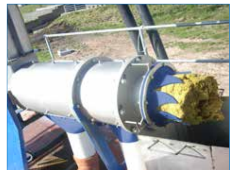
Slaughterhouse, cattle rumen (SEPCOM Industrial Horizontal)
