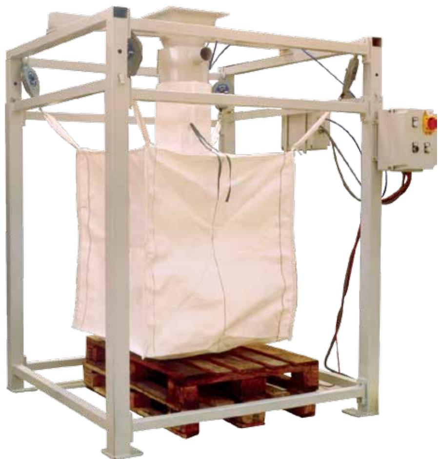
Suitable for filling FIBCs with material in powder or granular form. It comprises a supporting frame made of steel tubes containing two removable telescopic frames, which makes it possible to adapt the entire structure to different heights of FIBCs.
